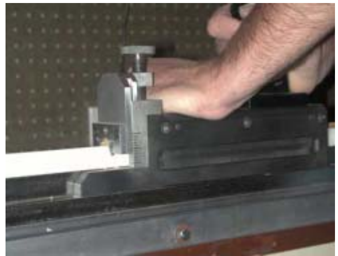
The Tom Morgan Rodsmith's Hand Mill has become one of the most innovative tools used by modern bamboo rodmakers.(photo courtesy of Tom Morgan and Gerri Carlson).
